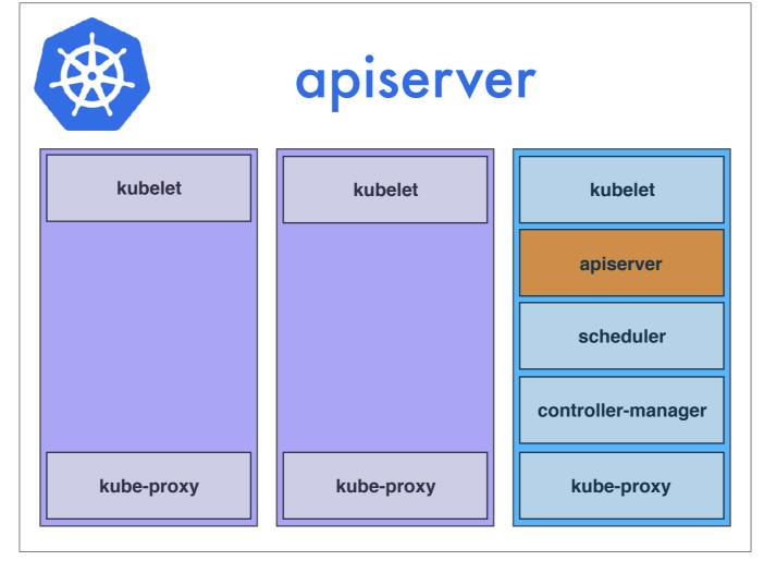
The API Server is the core of the k8s system. It handles validation of all the objects in the k8s cluster and acts as the frontend to the shared state, which is stored in etcd. If you want to inspect or alter Kubernetes managed objects, you do so through the apiserver.
