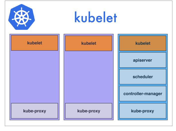
The most fundamental component of k8s is the Kubelet. This runs on every node in the cluster and has one main job. It takes manifests of containers you want to run on that node, and it makes sure they get run. The kubelet can actually stand alone. One way to provide containers to run is via the filesystem, and the kubelet will happily manage those for you without being part of a k8s cluster.
