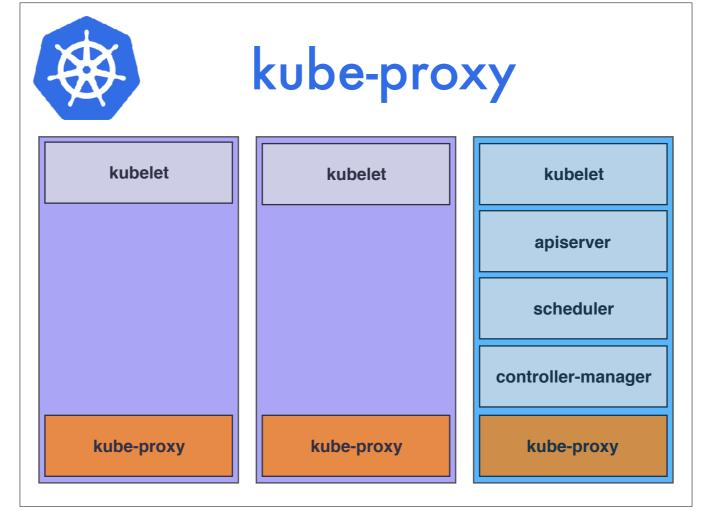
The kube-proxy is a service that runs on every node to provide a proxy for all of the services running in the cluster. This way, you can get routed to a node which can serve the service you're looking for without doing any special mapping in your application. This should become more clear later on.
