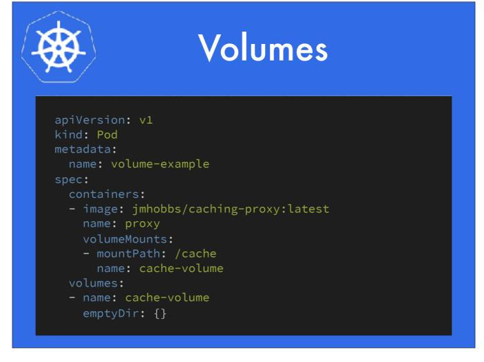
Here is an emptyDir. You can see it's definition at the very bottom there. An emptydir is a temporary directory that is created on the node when a pod is scheduled to it. When a pod is destroyed or removed from a node, the directory is too.
