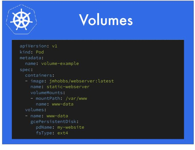
Sometimes you need storage that lasts. If you're on GCE, a Persistent Disk is ideal. These are not deleted after they are used like an emptyDir, so it can be passed around between pods with some coordination. These can also be mounted read only by multiple pods, which can be useful.
