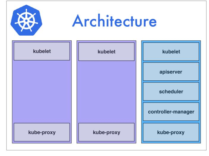
So this is a simplified overview of the architecture of Kubernetes. The purple boxes are worker nodes, these are the servers where your applications will be run. The blue box is a master node, which does not get work scheduled to it by default, and runs the software that coordinates the cluster and distributes work.
