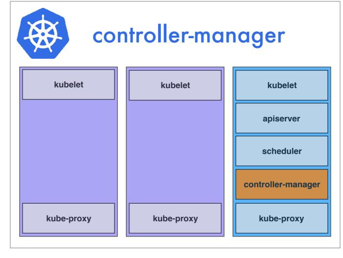
In k8s, a Controller is a loop which watches the state of the cluster through the apiserver and makes changes in an effort to move the current state towards the desired state. Examples being the service controller, node controller, etc. This is the engine of Kubernetes orchestration.
