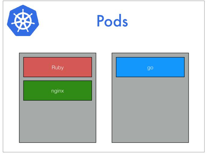
The most foundational object in k8s is the Pod. A Pod is a logical wrapper around one or more Docker containers. It is the indivisible unit of work.
